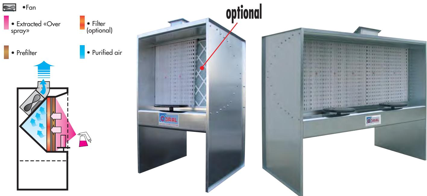
Suitable for painting small pieces, for small series or final touches. Available in two models (1 and 2 m), with fans fitted with a high-performance backward inclined spark proof impeller and a revolving part holder. They are supplied fitted with a paper filter; a further filtering stage made of glass fibre is available on request.
